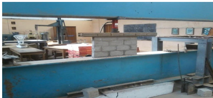
Figure 3. Test Set-up for masonry wallets compressive strength.
