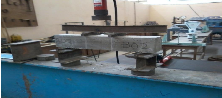
Figure 1. Set up for flexural tensile strength test.
