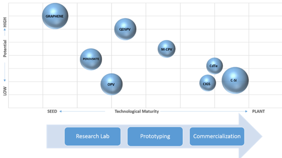
Figure 6. Potential Vs technological maturity for PV technologies.
