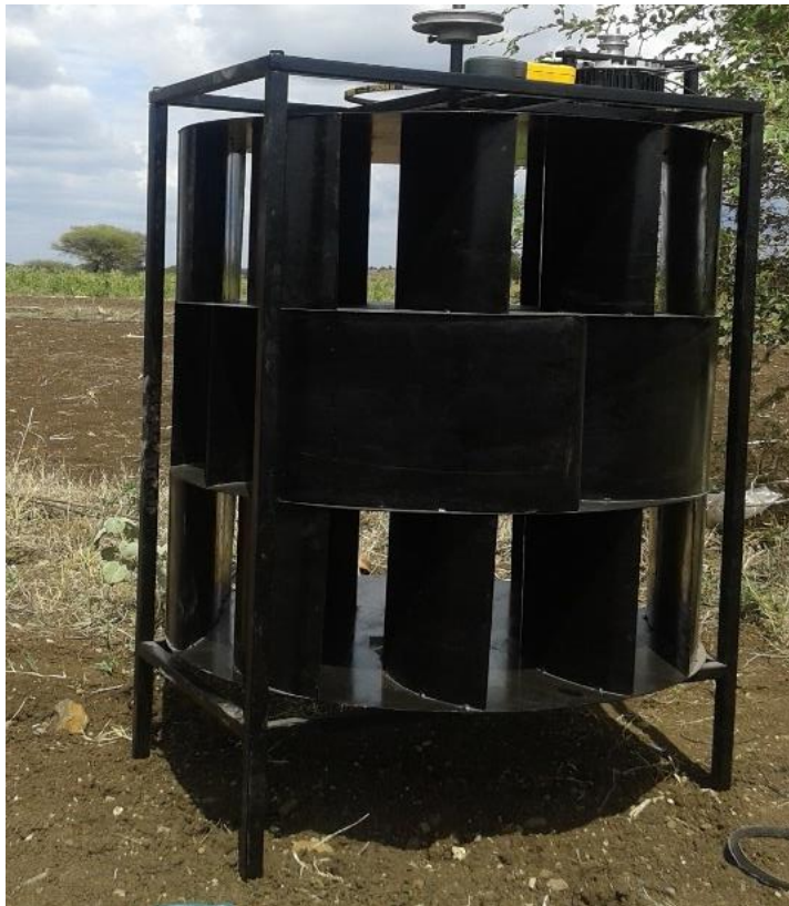
Figure 3. Model of threestorey Vertical Axis Wind Turbine.
