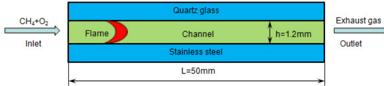
Fig. 2 Schematic diagram of the micro combustor structure with length 50 mm and height 1.2 mm.
