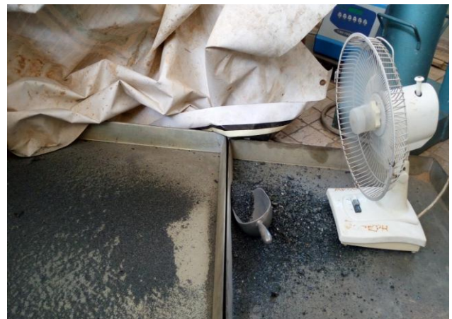
Fig. 2. Setup for winnowing process
