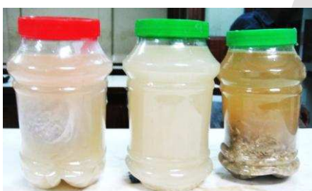
Fig. 3. i. HMCB OM ii. CES OM iii. HM OM Reaction mixtures of i. Gelatinised cassava starch and Obaatampa maize HMCB ii. Gelatinised cassava starch and Obaatampa maize CES iii. Gelatinised cassava starch and Obaatampa maize HM
