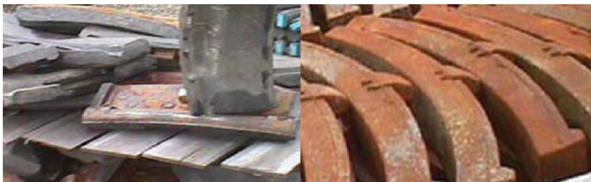
Figure 2. The cast brake shoes with wear indicators.
