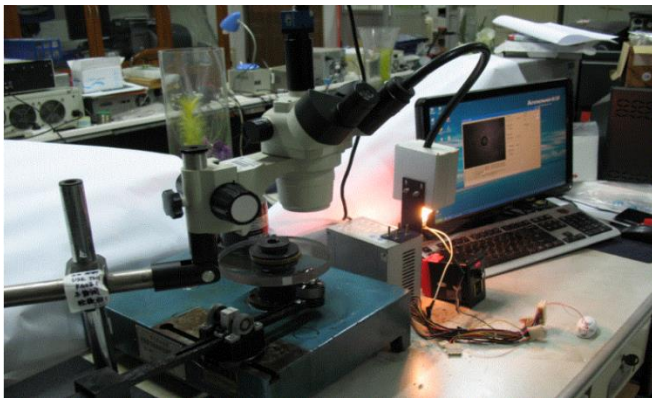
Figure 3 The setup of the optical interferometry image capturing.
